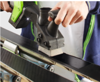
Melting head with larger contact surface
